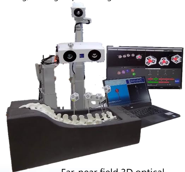
Far-near field 3D optical positioning system
